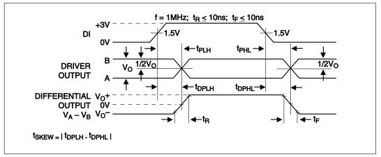
Figure 5. Driver Propagation Delays
