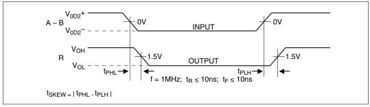
Figure 7. Receiver Propagation Delays
