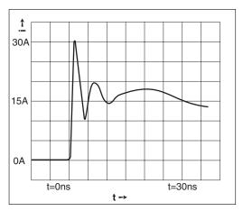
Figure 9. ESD Test Waveform for IEC1000-4-2
