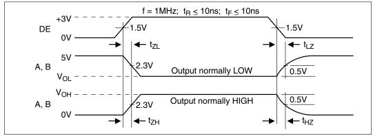
Figure 6. Driver Enable and Disable Times
