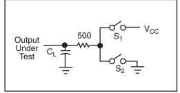
Figure 4. RS-485 Driver Timing Test Load #2 Circuit
