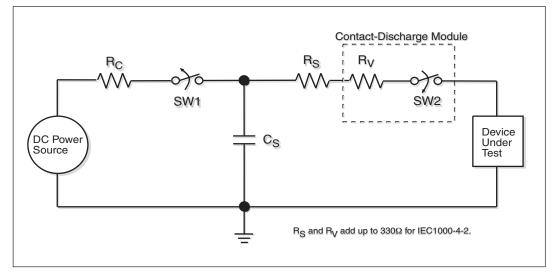
Figure 8. ESD Test Circuit for IEC1000-4-2
