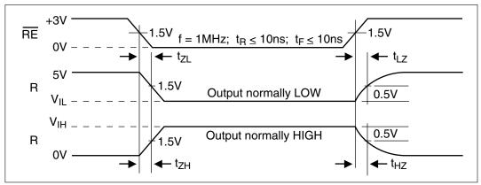
Figure 8. Receiver Enable and Disable Times
