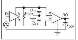
Figure 3. RS-485 Driver/Receiver Timing Test Circuit
