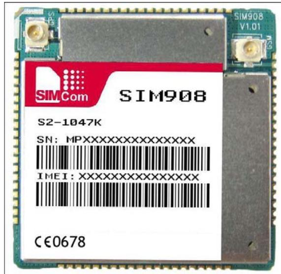
Figure 40: Top view of SIM908
