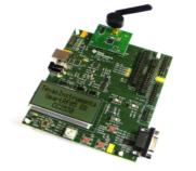
Make sure that P14 (the RS232 switch) is set in position *Enable* on this board.
