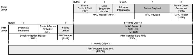
Figure 19-3. Schematic View of the IEEE 802.15.4 Frame Format [1]
