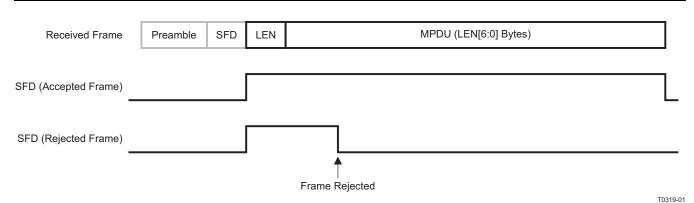
Figure 19-9. SFD Signal Timing
