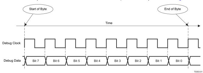
Figure 3-2. Transmission of One Byte
