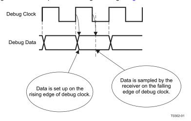
Figure 3-1. External Debug Interface Timing
