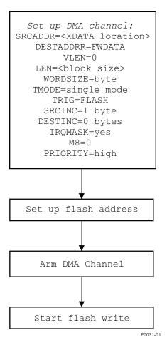
Figure 6-1. Flash Write Using DMA
