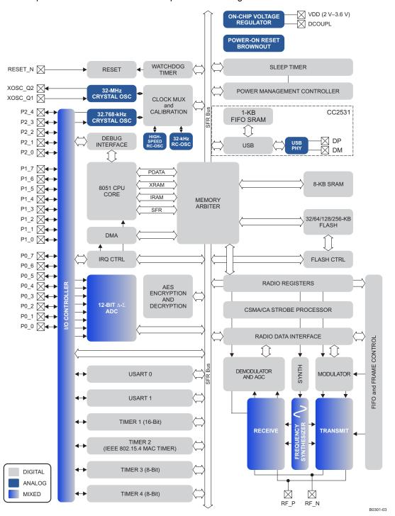
Figure 1-1. CC253x Block Diagram
