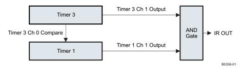
Figure 9-7. Block Diagram of Timers in IR-Generation Mode
