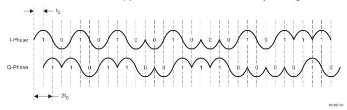
Figure 19-2. I/Q Phases When Transmitting a Zero-Symbol Chip Sequence,  $t_C = 0.5 \mu s$
