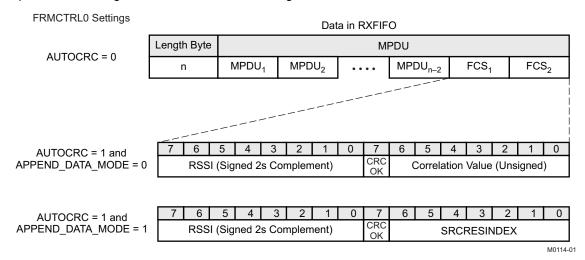
Figure 19-13. Data in RX FIFO for Different Settings
