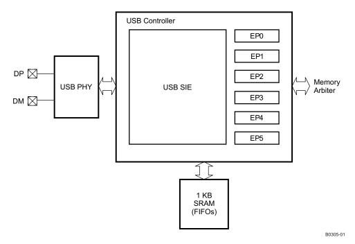
Figure 17-1. USB Controller Block Diagram
