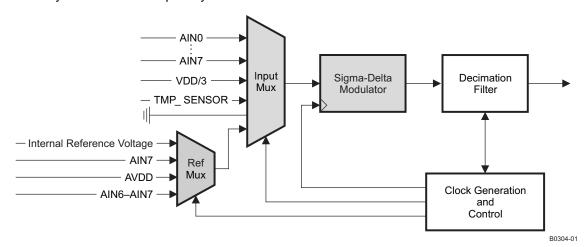
Figure 12-1. ADC Block Diagram
