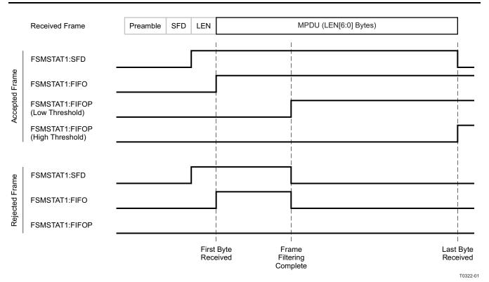
Figure 19-17. Behavior of FIFO and FIFOP Signals
