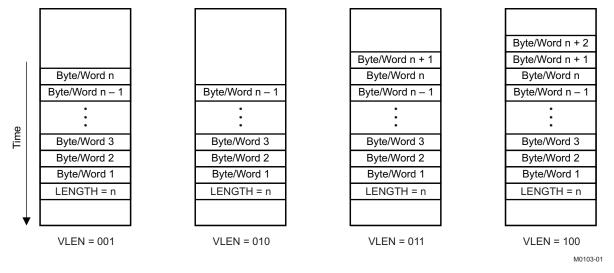
Figure 8-2. Variable Length (VLEN) Transfer Options
