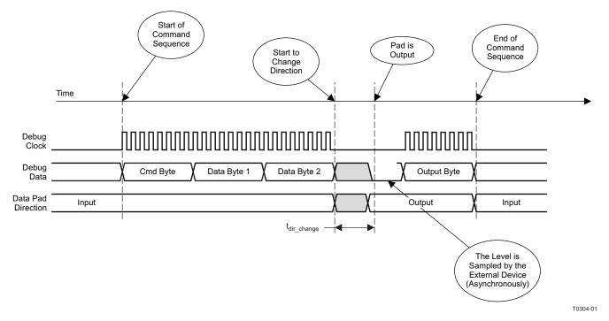
Figure 3-3. Typical Command Sequence—No Extra Wait for Response
