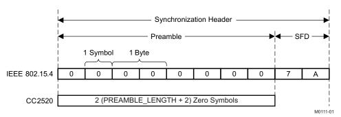
Figure 19-7. Transmitted Synchronization Header
