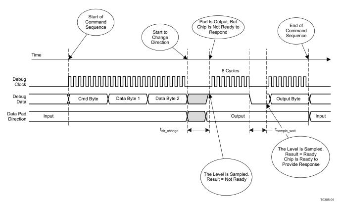
Figure 3-4. Typical Command Sequence. Wait for Response
