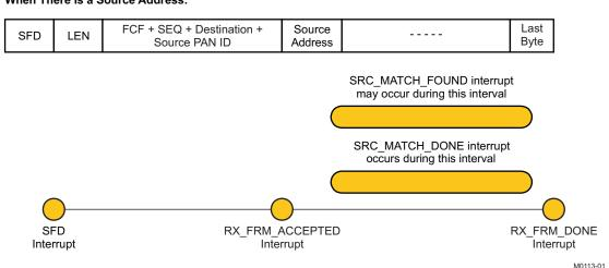
Figure 19-12. Interrupts Generated by Source Address Matching
