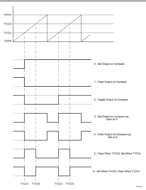
Figure 9-4. Output Compare Modes, Timer Free-Running Mode
