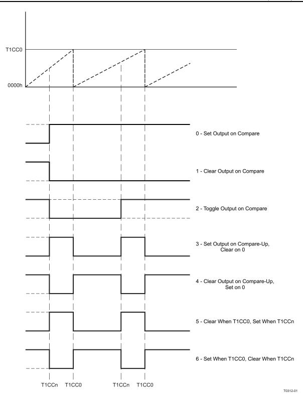
Figure 9-5. Output Compare Modes, Timer Modulo Mode
