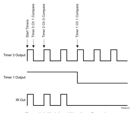
Figure 9-8. Modulated Waveform Example
