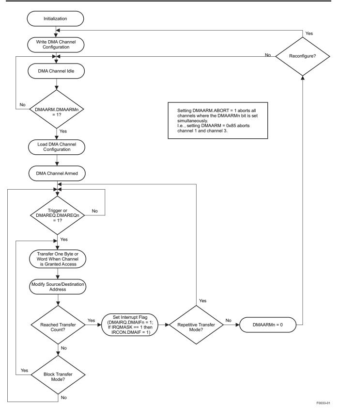
Figure 8-1. DMA Operation
