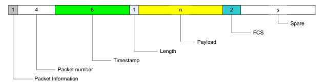
Figure 22: Packet format in PSD file
