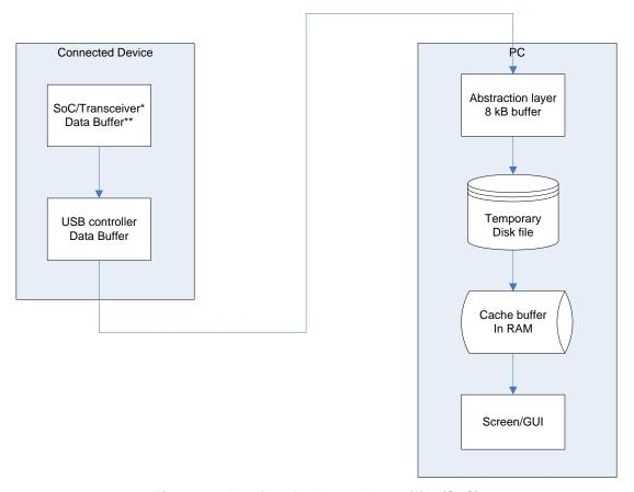
Figure 10: Dataflow for the packet sniffer (SoC)
