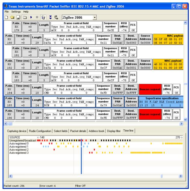
Figure 12: Packet sniffer screenshot from the IEEE8022.15.4/ZigBee protocols
