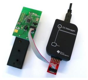
Figure 7: CC Debugger + SmartRFCCxx10TB
