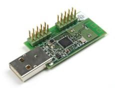
Figure 5: CC2511/CC1111 USB Dongle
