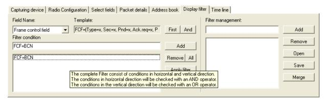
Figure 24: Display filter panel with the tool-tip shown
