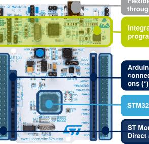
Flexible board power supply through USB or external source
