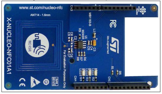
Figure 2. X-NUCLEO-NFC01A1 M24SR expansion board
