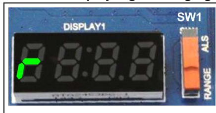
Figure 13. Left display digit in ranging mode
