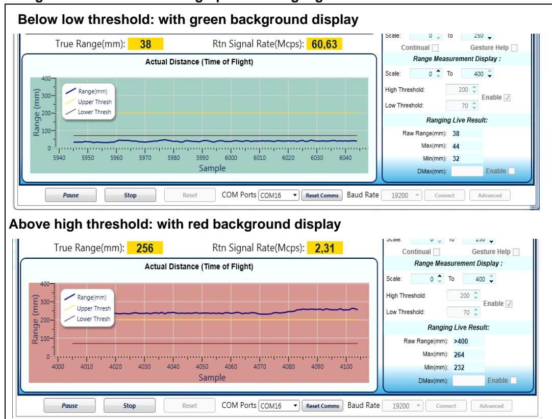
Figure 39. Actual distance graphs showing high and low thresholds
